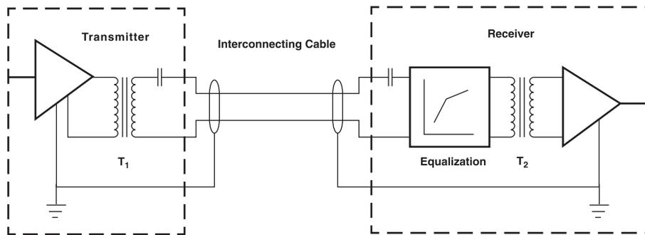
T<sub>1</sub>, T<sub>2</sub>: PE-65612 or PE-65812
