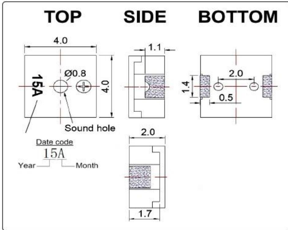
Tolerance:  $\pm 0.5\text{mm}$  except specified
