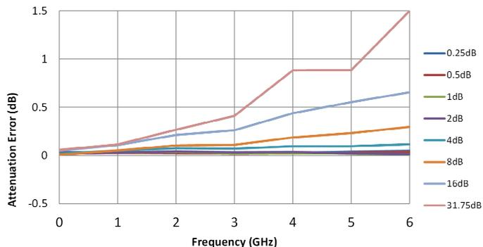
Figure 10. 0.25 dB Attenuation Error vs. Frequency
