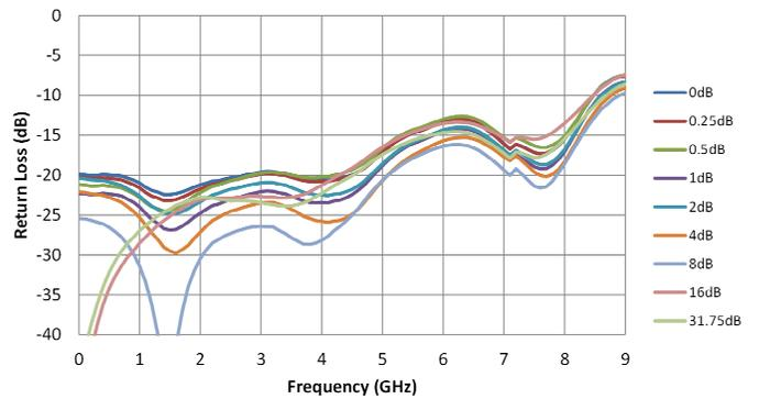
**Figure 21. Output Return Loss vs. Attenuation Setting**
