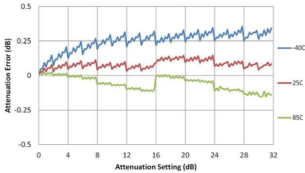
**Figure 27. Attenuation Error @ 1800 MHz vs. Temperature**
