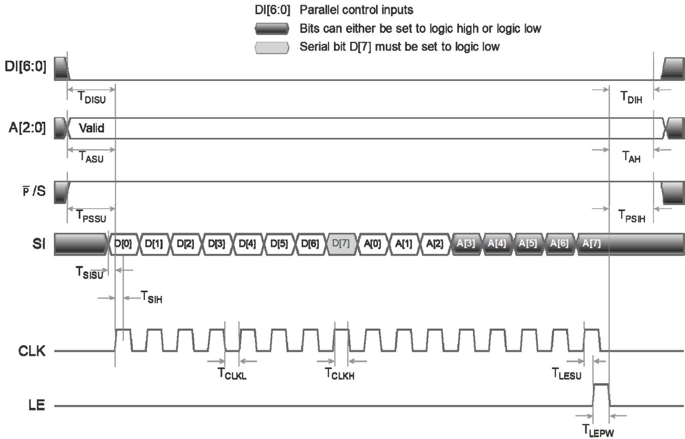
Figure 6. Latched-Parallel/Direct-Parallel Timing Diagram
