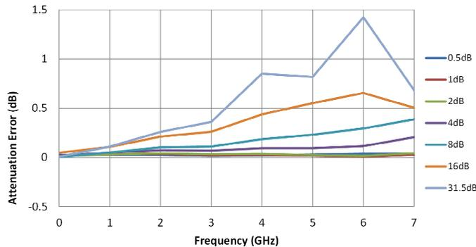
**Figure 14. 0.5 dB Attenuation Error vs. Frequency**
