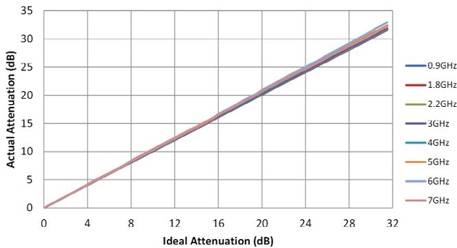
**Figure 13. 0.5 dB Major State Bit Error vs. Attenuation Setting**
