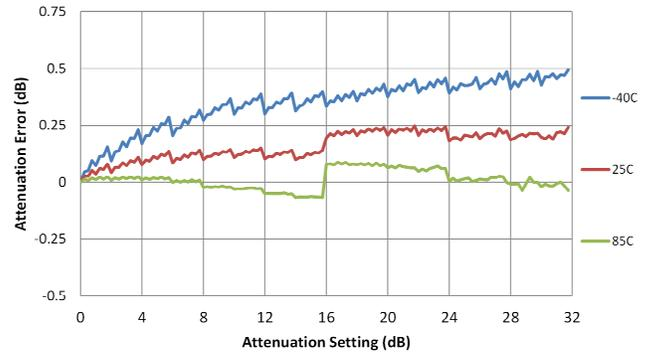
**Figure 28. Attenuation Error @ 3000 MHz vs. Temperature**
