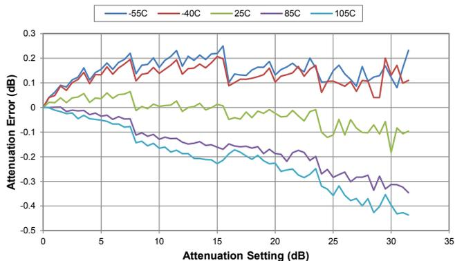
Figure 20. Attenuation Error @ 100 MHz vs Temperature
