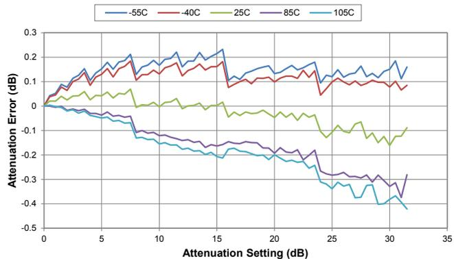
Figure 21. Attenuation Error @ 1 GHz vs Temperature
