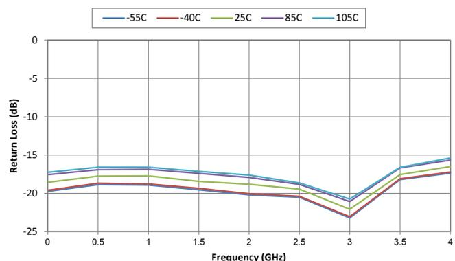
Typical Performance Data @ 25 °C and  $V_{DD} = 3.3V$ , unless otherwise noted
