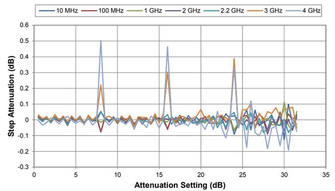
Note: \* Monotonicity is held as long as step attenuation does not cross below - 0.5 dB.
