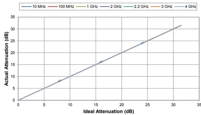
Figure 16. 0.5 dB Step Attenuation vs Attenuation Setting\*
