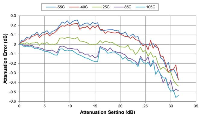
Figure 23. Attenuation Error @ 4 GHz vs Temperature
