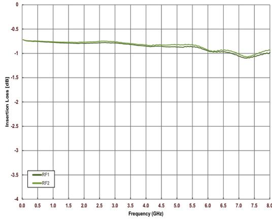
Figure 3 ■ Insertion Loss vs. Temp (RFC–RFX)
