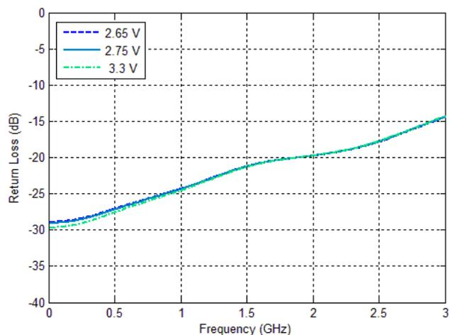
Figure 8. Return Loss vs Temp (Common Port)
