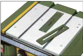
Non-slotted sawing gap cover of ABS for tight tolerances between saw blade and table (is slotted from below by the FET saw blade). For cutting very small parts.
