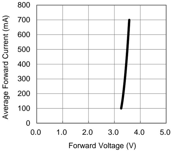
Fig 1. Forward Current vs. Forward Voltage for UV-M.
