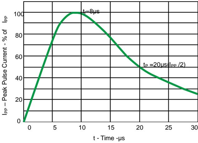
Fig 1. Pulse Waveform
