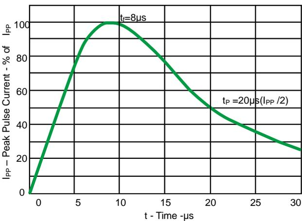
Fig 1.Pulse Waveform
