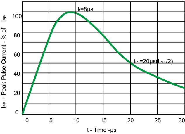
Fig 1. Pulse Waveform
