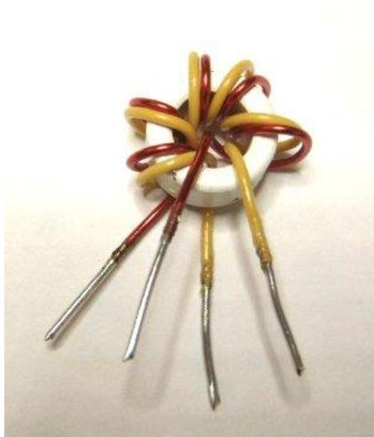
**Figure 19** – Finished Inductor.
