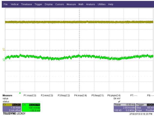
**Figure 61** – Output Ripple, Full Load, 39 V<sub>OUT</sub>, 115 VAC.
