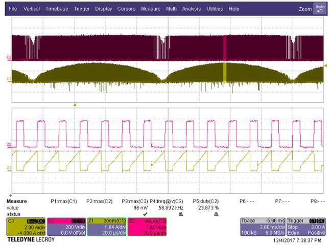
**Figure 46** – PFC Stage Drain Voltage and Current, Full Load, 115 VAC, 60 Hz.
