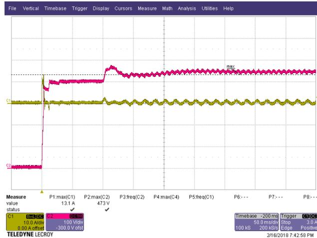
**Figure 52** – AC Input Current vs. PFC Output Voltage at Start-up, Full Load, 277 VAC, 60 Hz.
