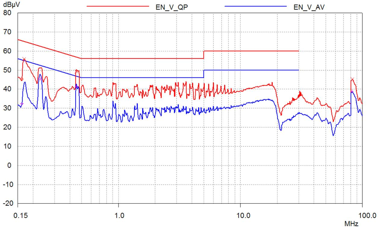
Figure 81 – Conducted EMI, 230 VAC, Full Load.
