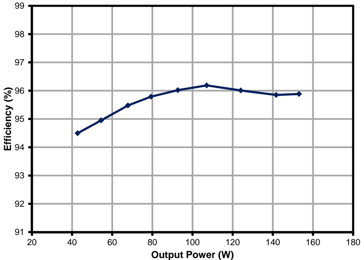
Figure 24 – LLC Stage Efficiency vs. Load, 380 VDC Input.
