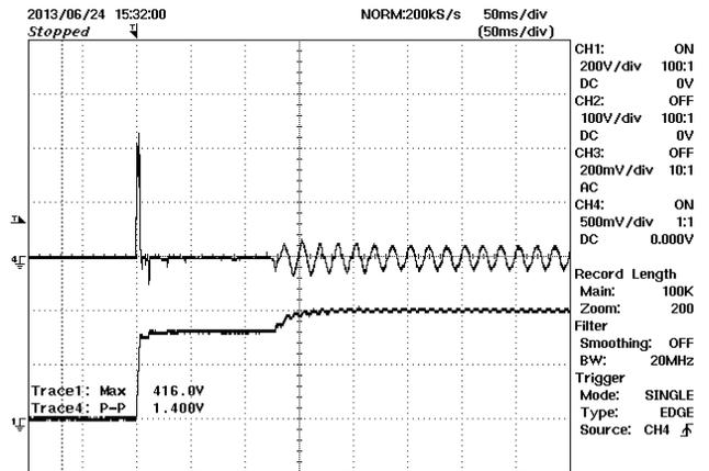
**Figure 41** – AC Input Current vs. PFC Output Voltage at Start-up, Full Load, 230 VAC.
