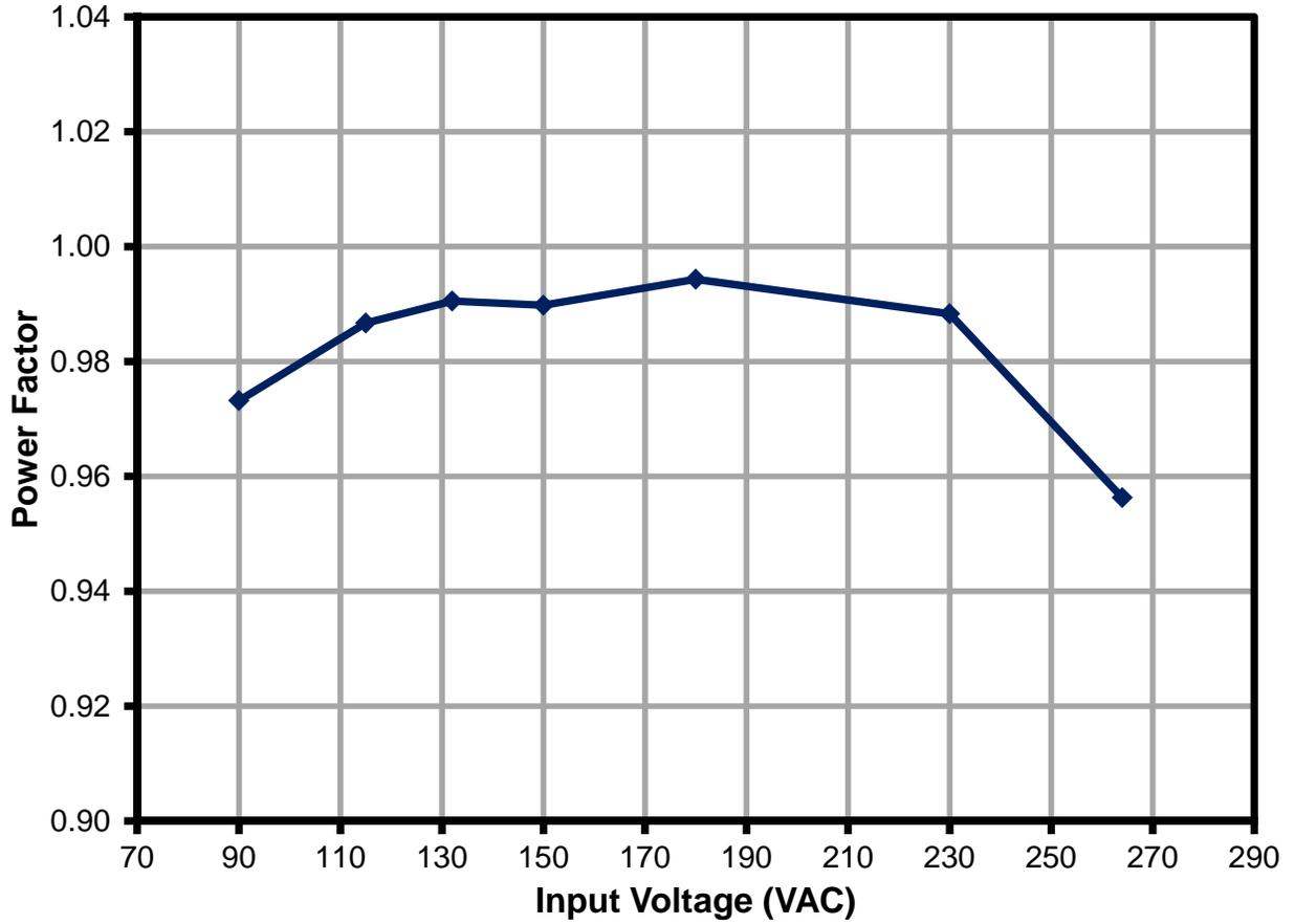
Figure 26 – Power Factor vs. Input Voltage, 100% Load.
