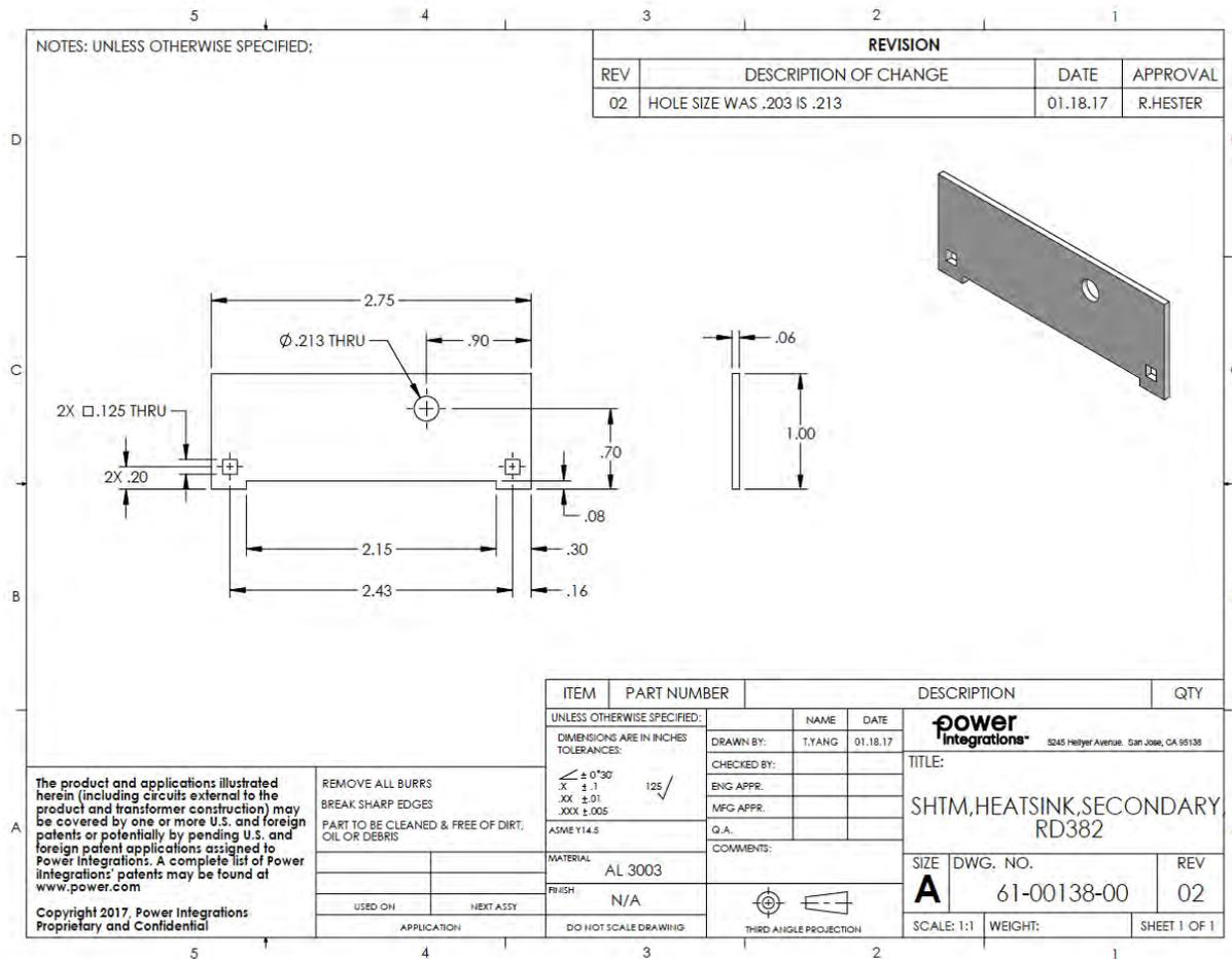
Figure 21 – Secondary Heat Sink Sheet Metal Drawing.
