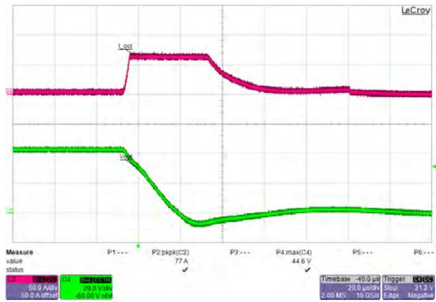
**Figure 45** – Output Short-Circuit Test.
