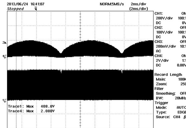
**Figure 38** – PFC Stage Drain Voltage and Current, Full Load, 230 VAC.
