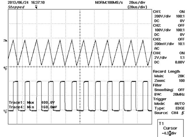
**Figure 37** – PFC Stage Drain Voltage and Current, Full Load, 115 VAC.
