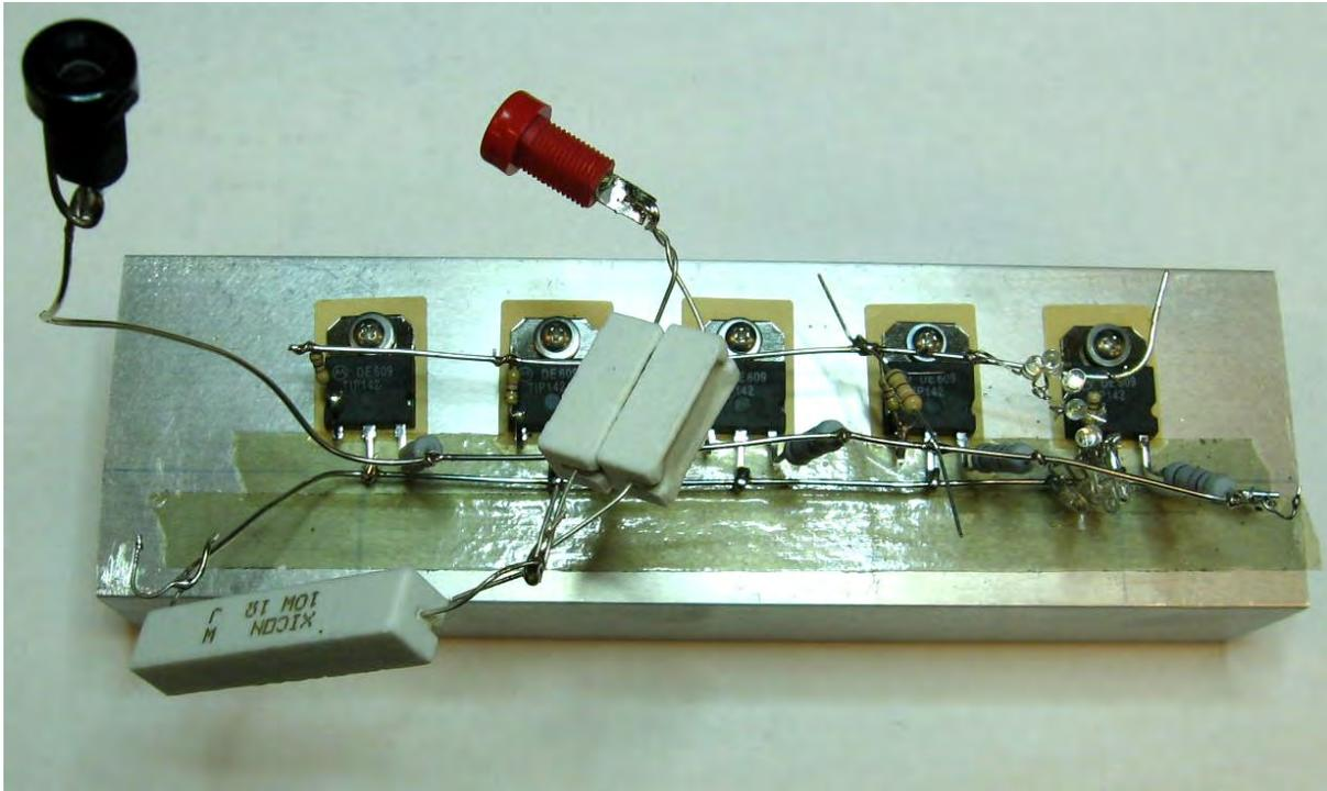
Figure 11 – Constant Voltage Load with Heat Sink.
