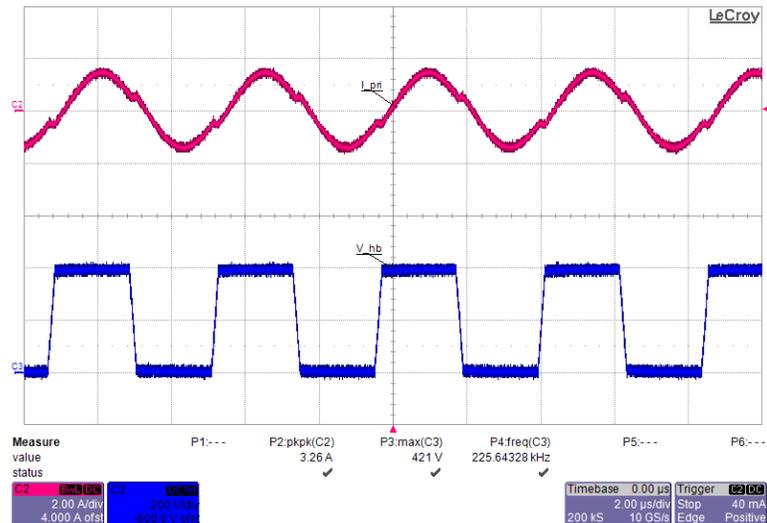
**Figure 33** — LLC Stage Primary Voltage and Current, 100% Load.
