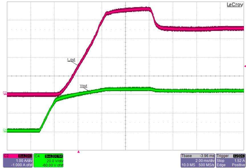
**Figure 43** – LLC Start-up. 115 VAC, 100% Load, LED Load.
