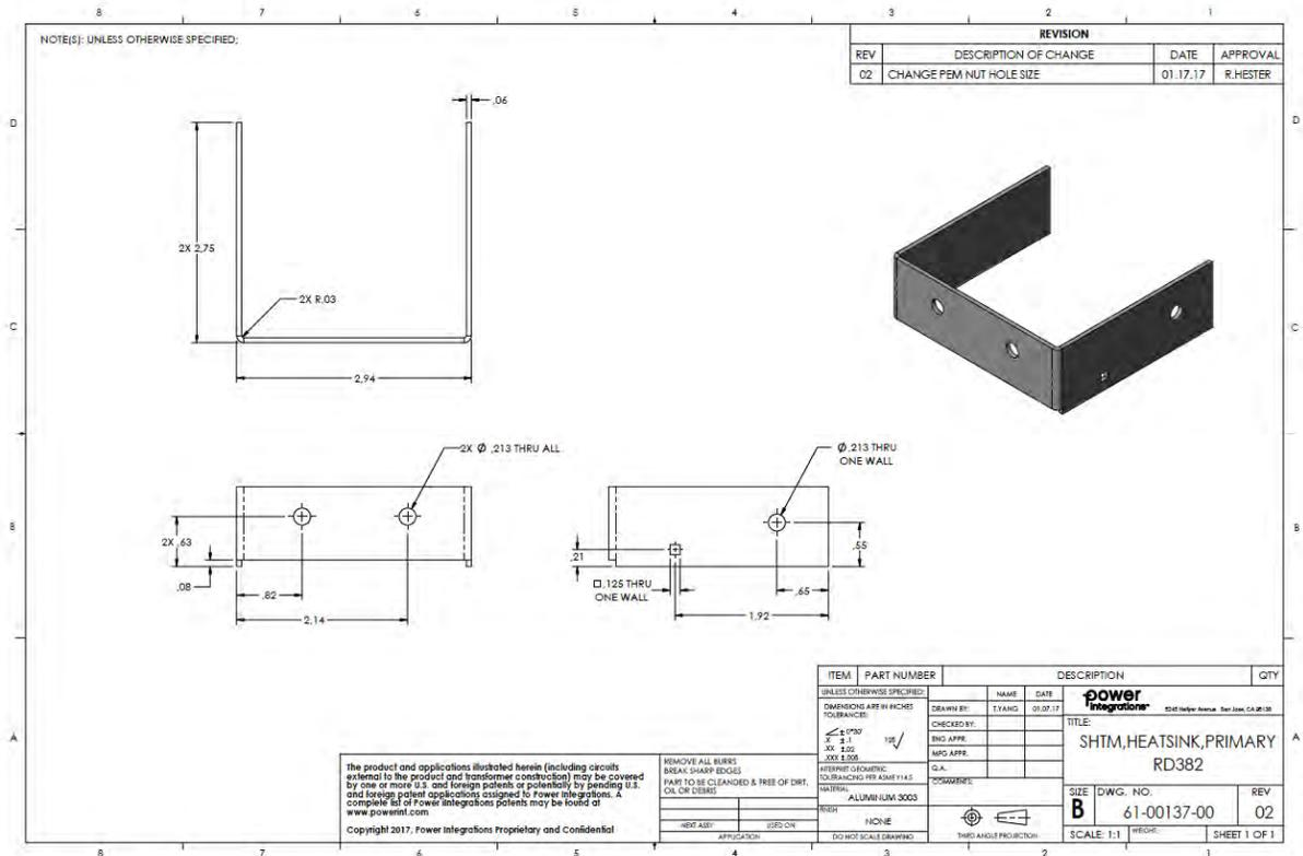
11.1.2 Primary Heat Sink with Fasteners
