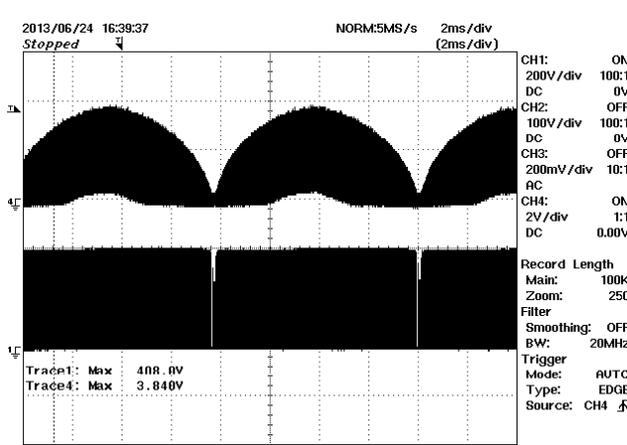
**Figure 36** – PFC Stage Drain Voltage and Current, Full Load, 115 VAC.
