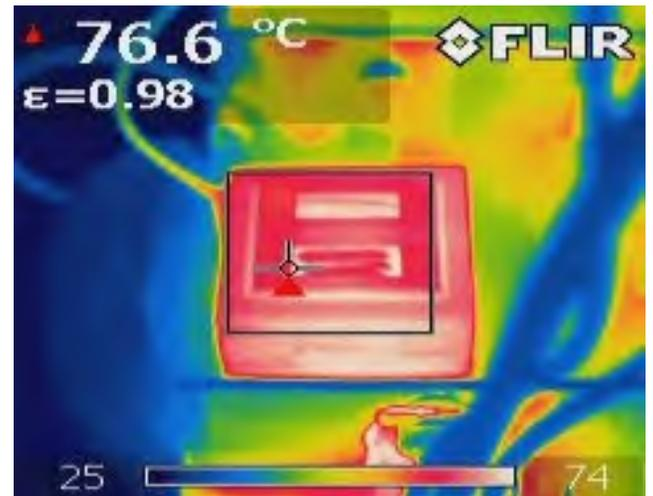
**Figure 66** – LLC Transformer (T1), 115 VAC Input, 100% Load, Room Temperature.
