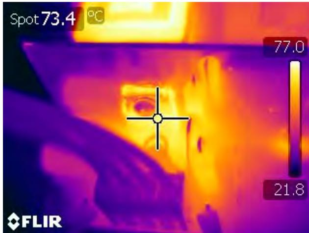
**Figure 77** – Output Rectifier (D11), 230 VAC Input, 100% Load, Room Temperature.
