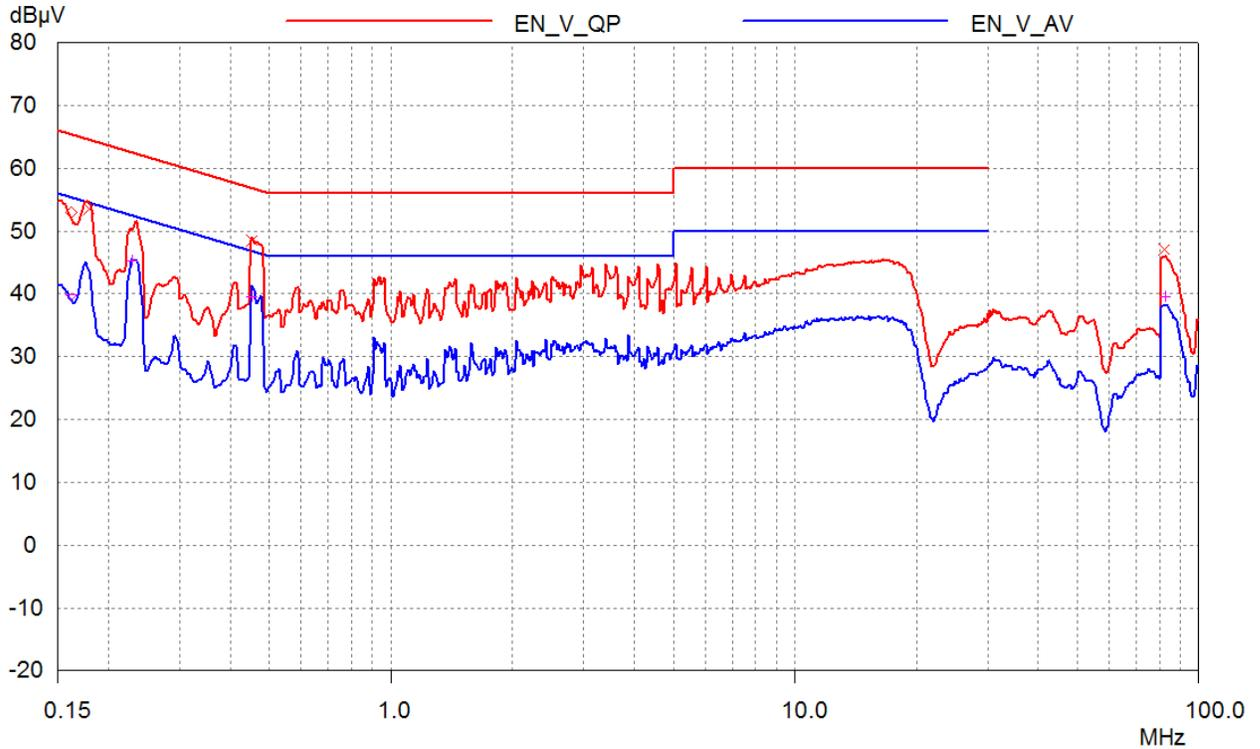
Figure 80 – Conducted EMI, 115 VAC, Full Load.
