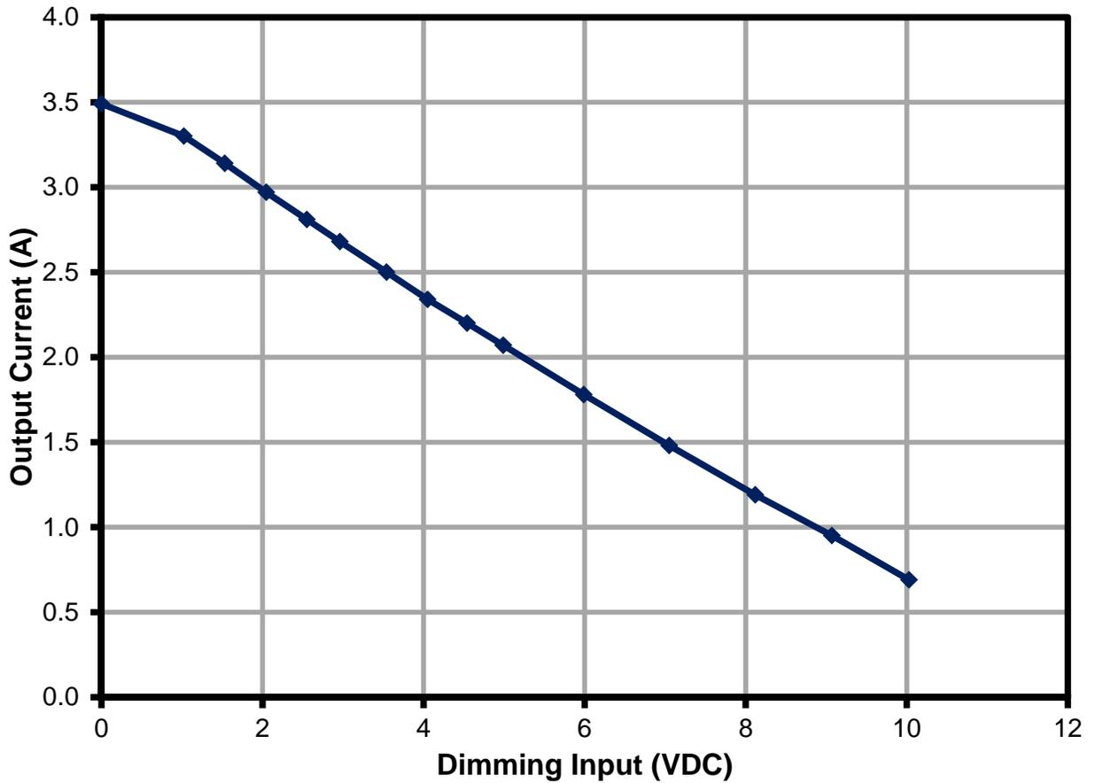
Figure 28 – RD-382 Output Current vs. Dimming Voltage.
