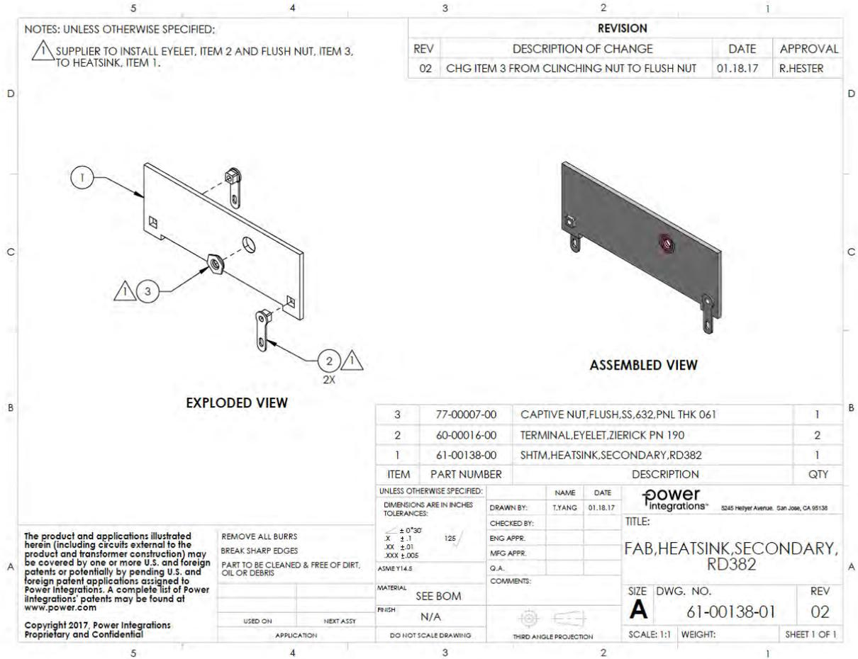
Figure 22 – Finished Secondary Heat Sink with Installed Fasteners.
