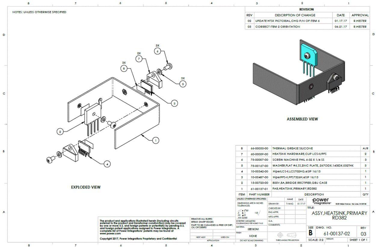
Figure 20 – RD-382 Primary Heat Sink Assembly.
