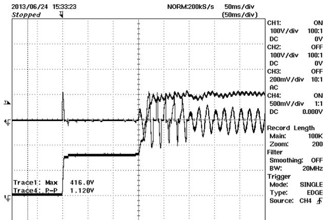
**Figure 40** – AC Input Current vs. PFC Output Voltage at Start-up, Full Load, 115 VAC.
