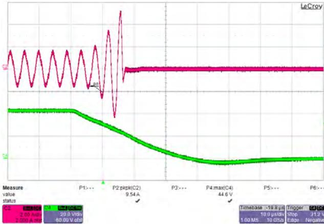
**Figure 44** – Output Short-Circuit Test.
