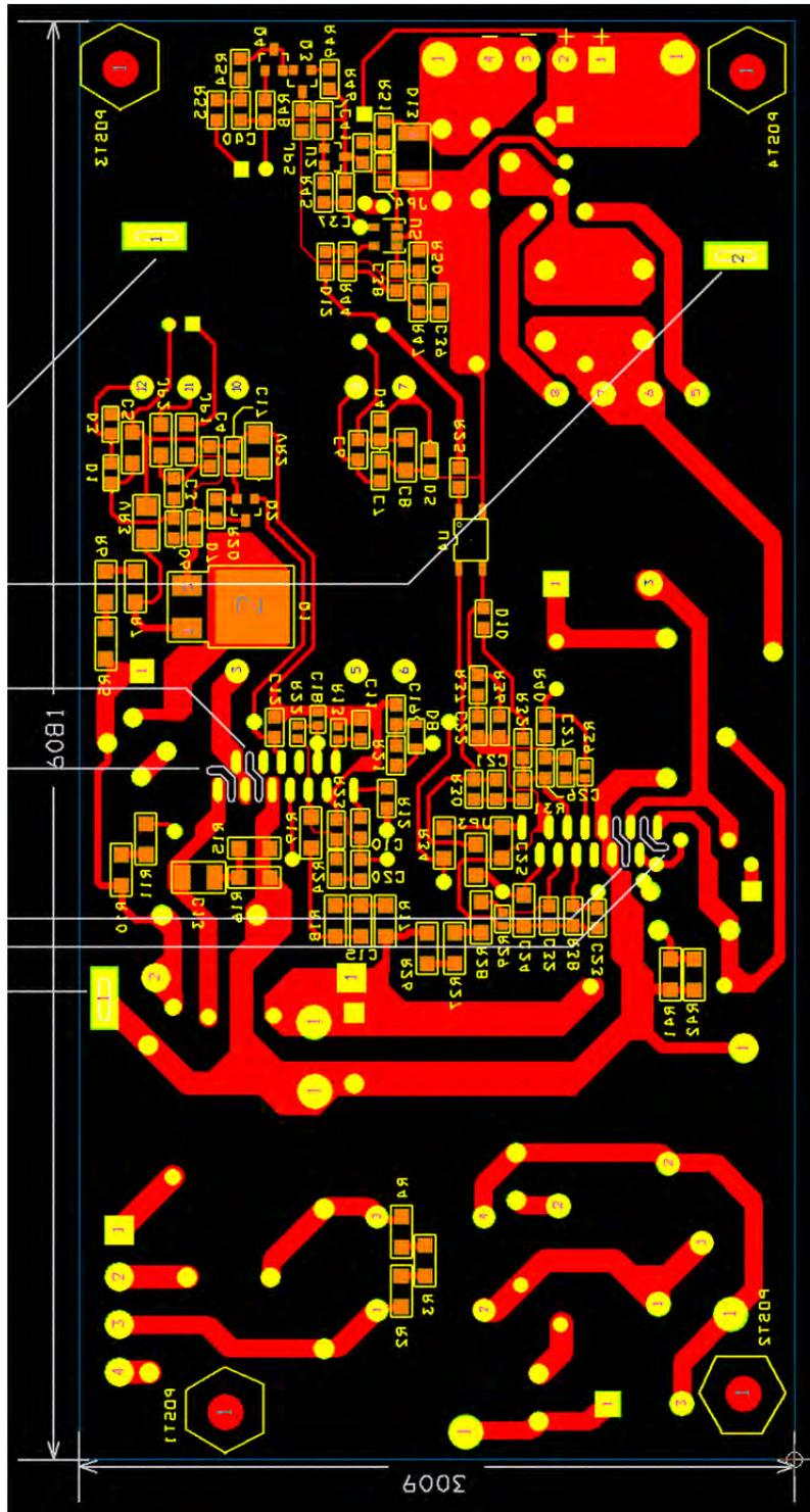
Figure 6 – Printed Circuit Layout, Bottom Side.
