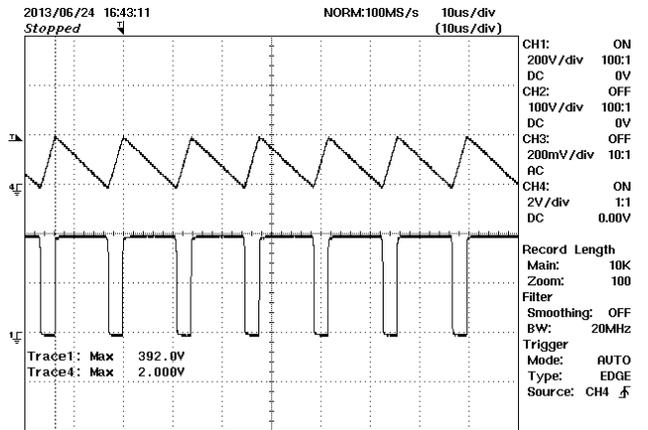
**Figure 39** – PFC Stage Drain Voltage and Current, Full Load, 230 VAC.
