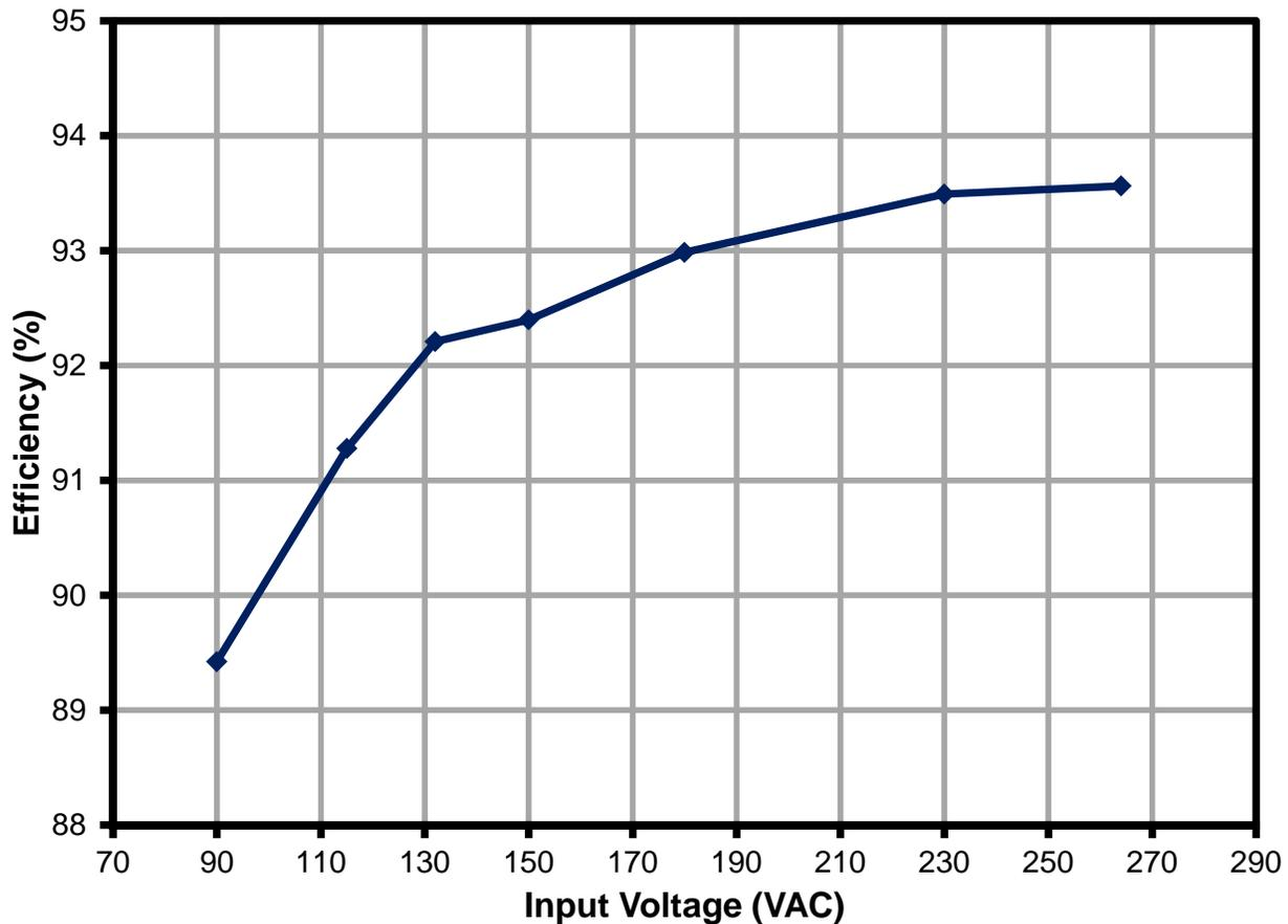
Figure 25 – Total Efficiency vs. Input Voltage, 100% Load.
