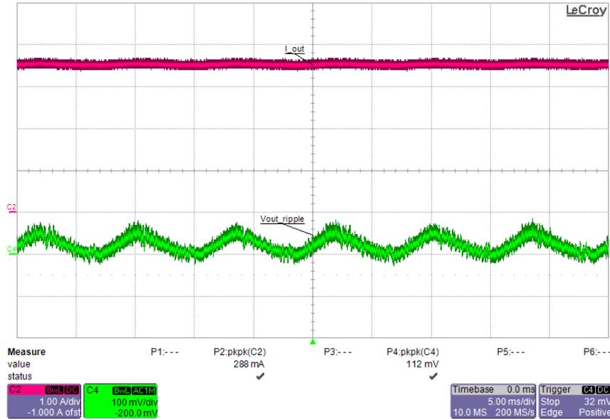
**Figure 48** – Output Ripple, Full Load, 115 VAC.
