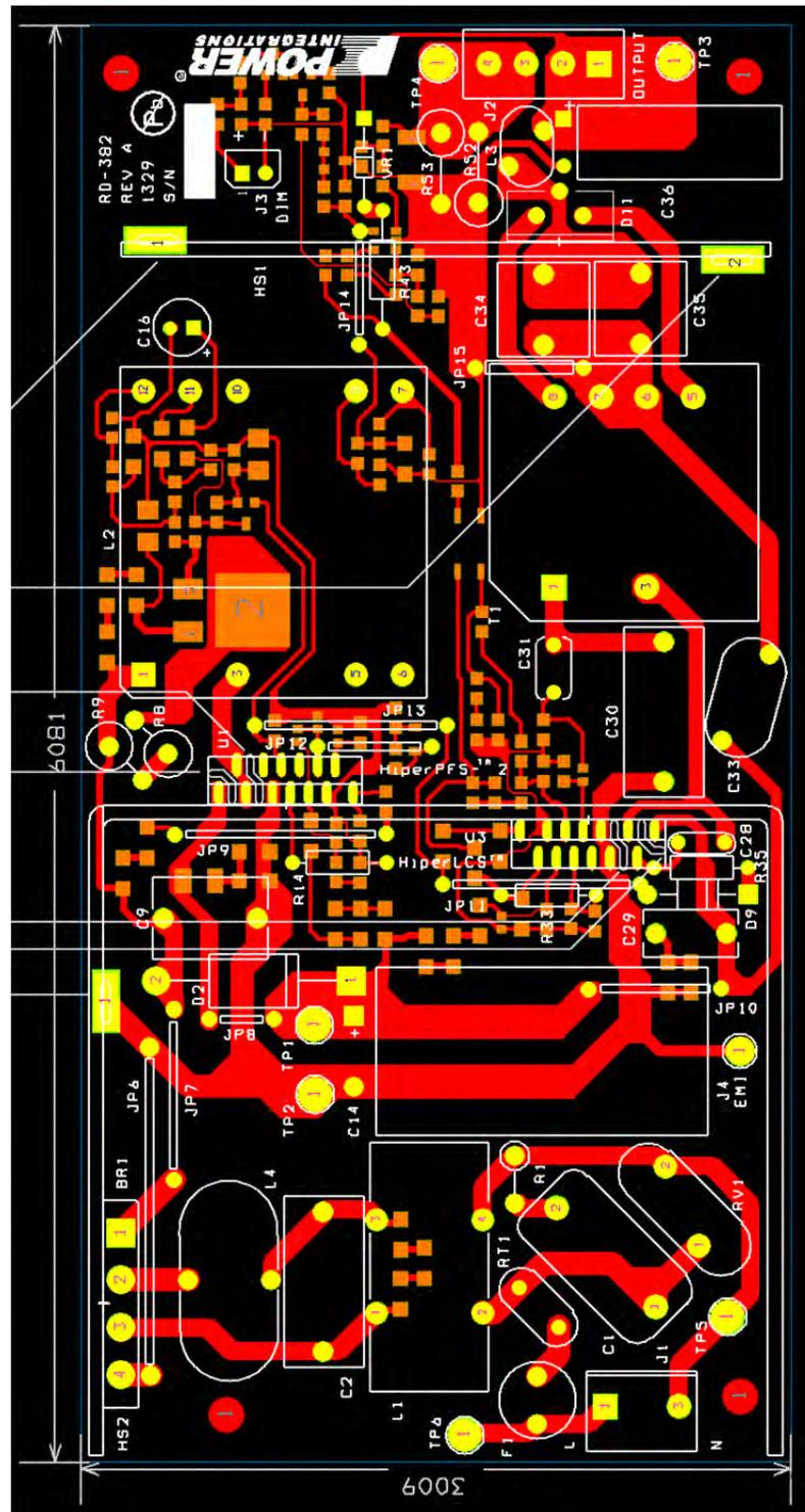
Figure 5 – Printed Circuit Layout, Top Side.
