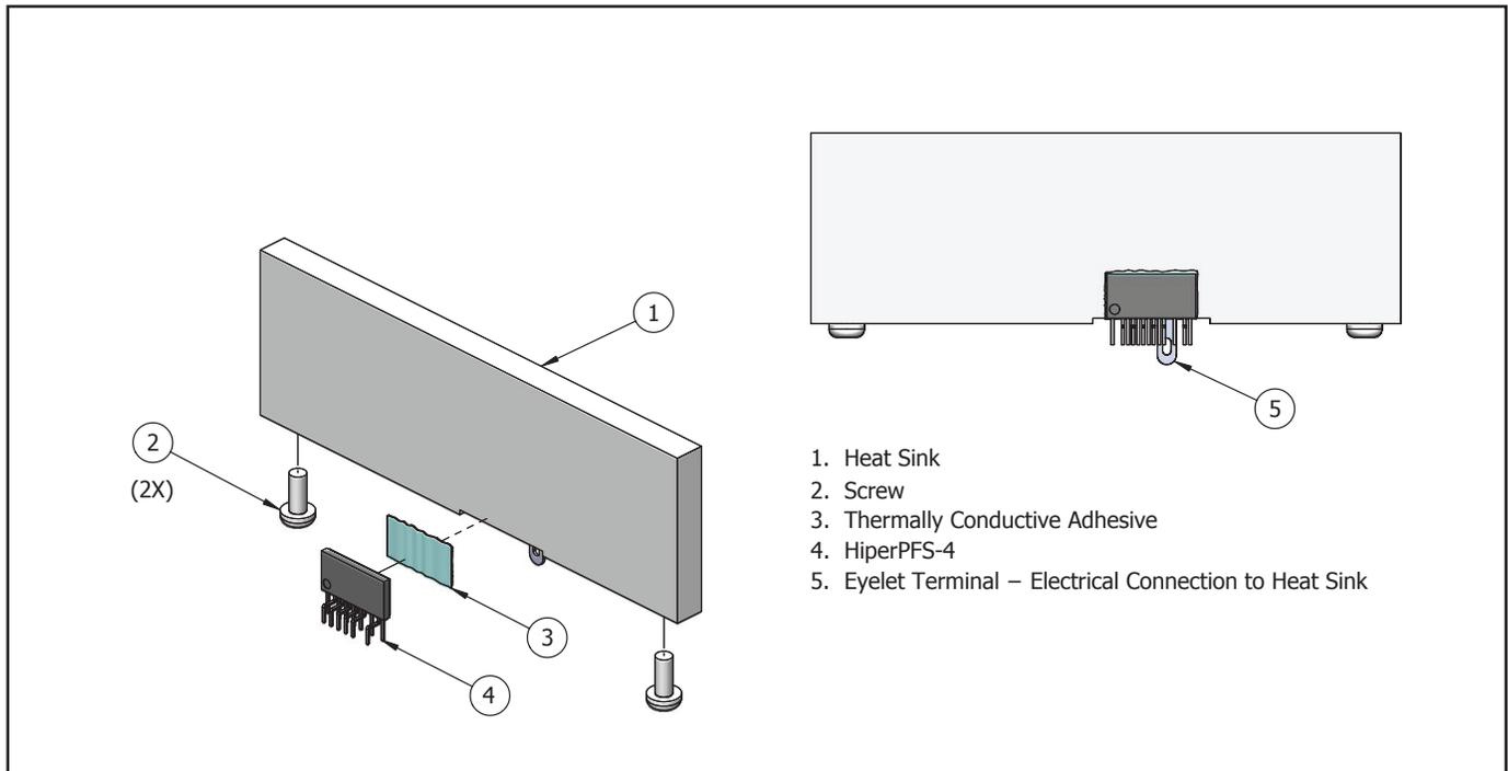
Figure 15. Heat Sink Assembly – using Thermally Conductive Adhesive.
