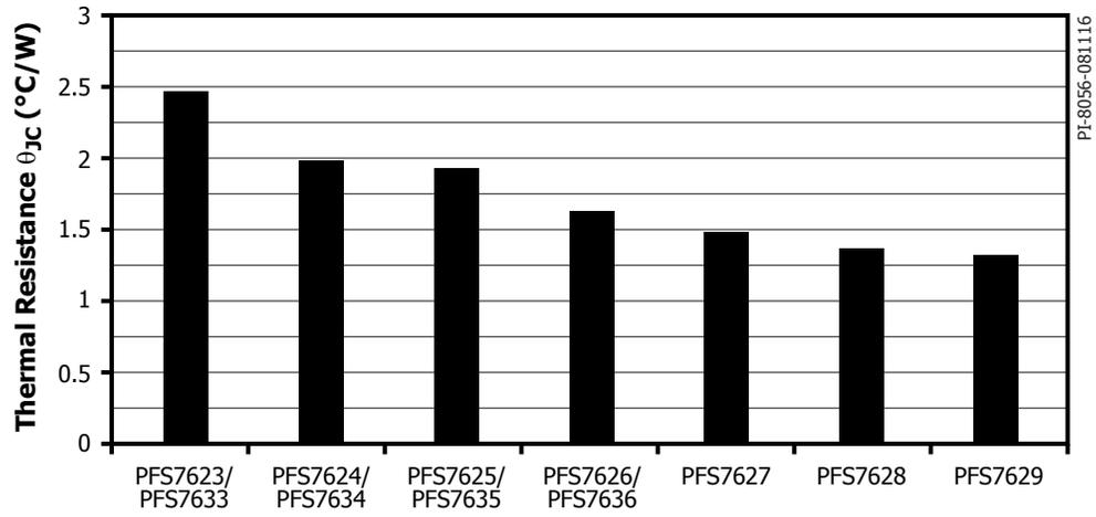
Figure 19. Thermal Resistance eSIP-16D / eSIP-16G Package ( $\theta_{Jc}$ ).
