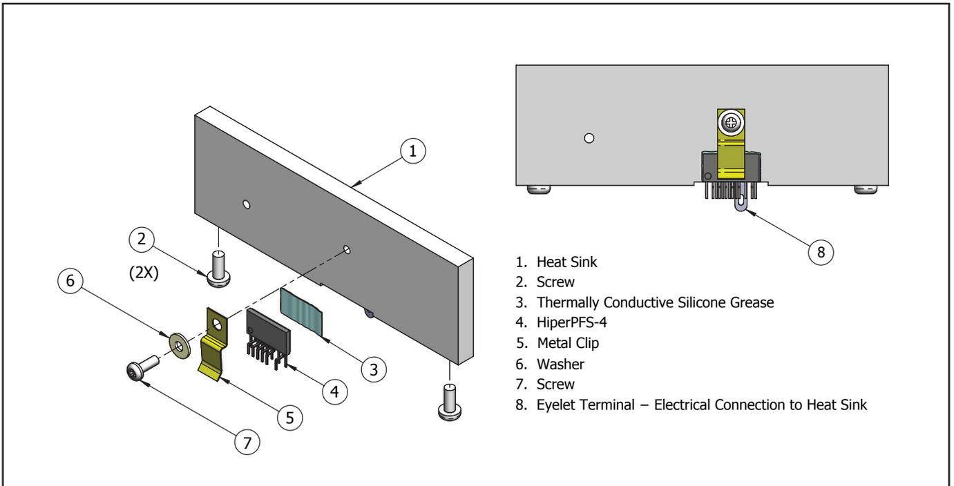
Figure 16. Heat Sink Assembly – with Metal Clip.
