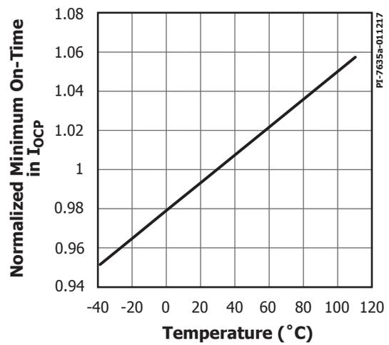
Figure 23. Normalized On-Time in IOCP vs. Temperature.
