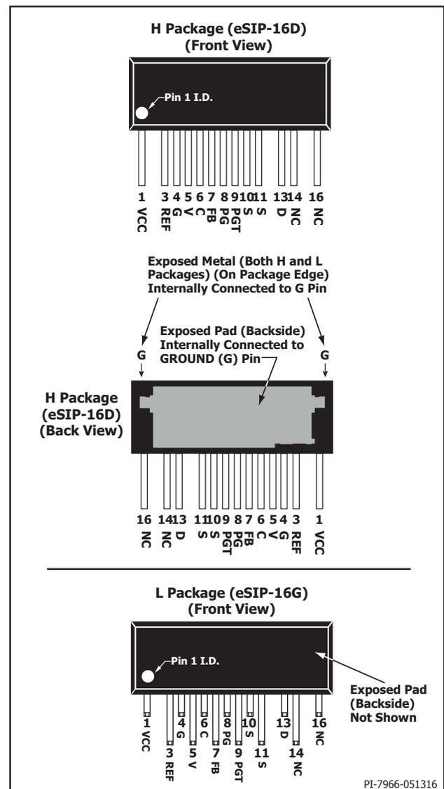
Figure 3. Pin Configuration.
