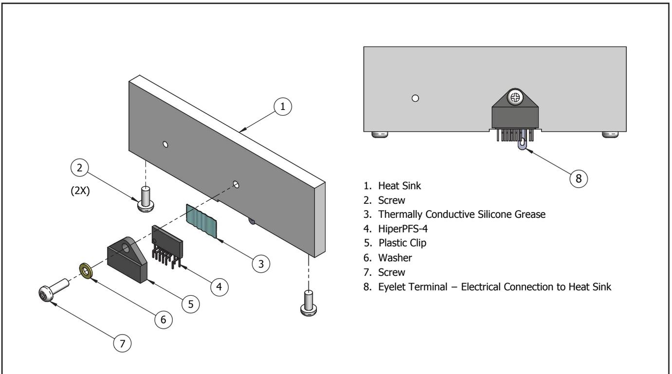
Figure 17. Heat Sink Assembly – with Plastic Clip.
