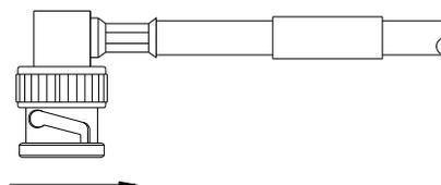
8. SLIDE INSULATOR INTO CONNECTOR AND SCREW NUT. SLIDE SHRINK TUBING OVER CRIMP AND SHRINK.
