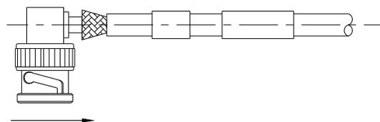
7. CRIMP OUTER FERRULE WITH APPROPRIATE CRIMP TOOL.
