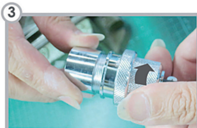
本體與上固定體對鎖，將螺紋順時針方向鎖緊（需轉動本體鎖入，非轉動接頭） The body and the upper one are locked together. Screw clockwise and be sure to only rotate the body itself instead of the whole connector
