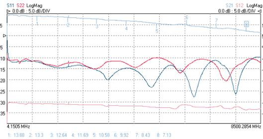
Show all S-parameters separately or combine on a single plot. Configure as one, two or four channels and show one to four live traces on each. Add one to four memory traces to each.
