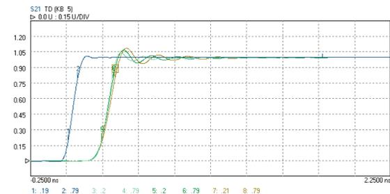
Compare network pulse responses using  $S_{21}$  time domain. Here using a live trace and up to four memory traces to compare low pass filter responses with through response.
