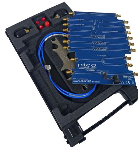
PCA includes example attenuator, broadband amplifier, 25  $\Omega$  mismatched line, resistive power divider, lowpass and bandpass filters and a user chip component site, plus short, open, load and through calibration elements.
