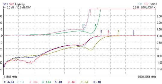
Plot both reflection parameters ( $S_{11}$ ,  $S_{22}$ ) as LogMag and SWR. Two of four memory traces in use to compare another DUT.
