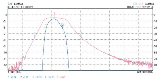
Display a single parameter at two sensitivities or offsets. Here we see passband  $S_{21}$  flatness and  $S_{21}/S_{12}$  stopbands as live traces on the same plot.
