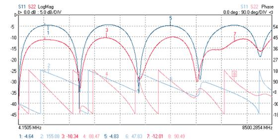
Plot both reflection parameters ( $S_{11}$ ,  $S_{22}$ ) as LogMag and Phase. Gain and phase can be combined in one plot, but with up to four live traces, why not plot forward and reverse match and gain and phase together, as above?
