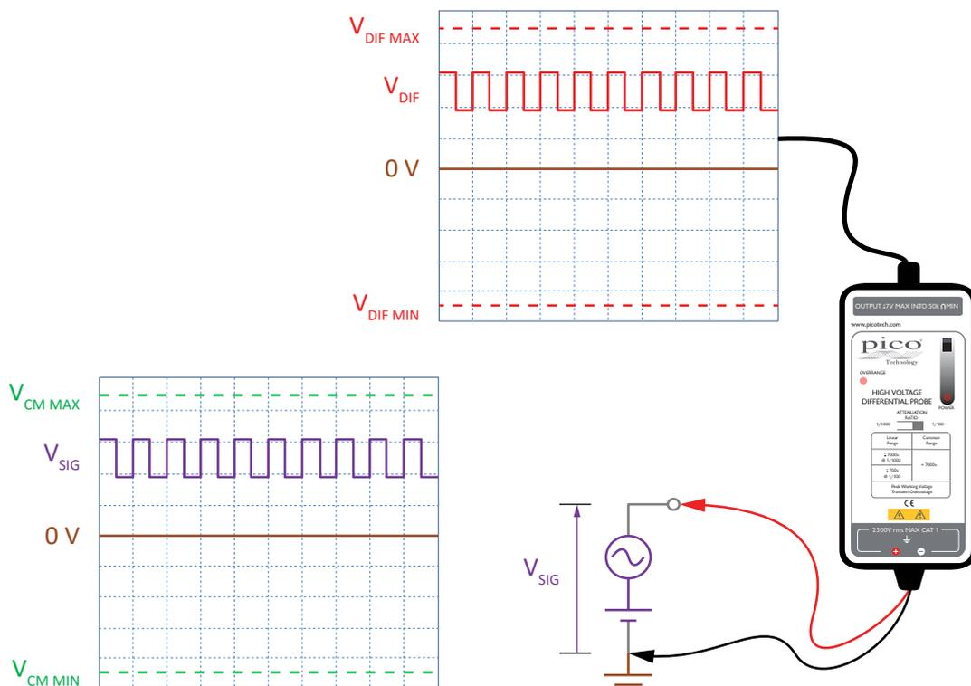
Figure 3 - Single-ended measurement
