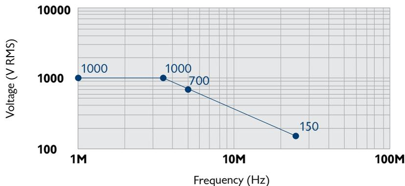
In the example above, the absolute maximum voltage on either of the inputs at low frequencies is 1000 V RMS. At about 3.3 MHz the voltage starts to decline, until at about 25 MHz it is only 150 V RMS. In practice this is seldom a limitation as high frequency and high voltage are rarely found together – such signals being more challenging to generate than they are to measure.
