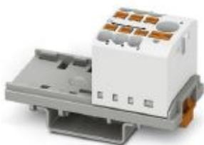
Distribution block, Block with vertical alignment and integrated supply, The blocks can be bridged with one another via the conductor shaft. For corresponding plug-in bridges, see accessories, nom. voltage: 690 V, nominal current: 24 A, connection method: Push-in connection, Push-in connection, number of connections: 7, cross section: 0.14 mm<sup>2</sup> - 4 mm<sup>2</sup>, AWG: 26 - 12, width: 28.6 mm, color: white, mounting type: NS 35/7,5, NS 35/15
