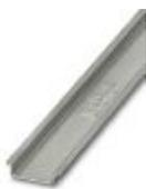
DIN rail, unperforated, Standard profile, width: 35 mm, height: 7.5 mm, acc. to EN 60715, material: Steel, galvanized, passivated with a thick layer, length: 2000 mm, color: silver
