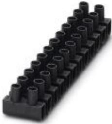
Polypropylene Europe terminal strip, black, for connecting solid conductors and stranded conductors with and without ferrules with a cross section of 0.75 to 6 mm<sup>2</sup>
