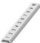
Zack Marker strip, flat, Strip, white, labeled, printed horizontally: consecutive numbers 1 ... 10, 11 ... 20, etc. up to 491 ... 500, mounting type: snap into flat marker groove, for terminal block width: 5 mm, lettering field size: 5.15 x 5.15 mm, Number of individual labels: 10
