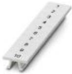
Zack marker strip, white, Printed vertically: consecutive numbers 1 ... 10, 11 ... 20, etc. up to 491 ... 500, mounting type: snap into tall marker groove, for terminal block width: 5.2 mm, lettering field size: 5.15 x 10.5 mm
