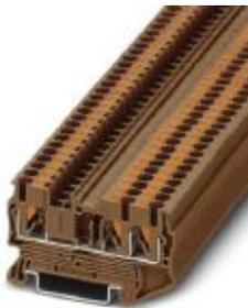
Feed-through terminal block, nom. voltage: 800 V, nominal current: 24 A, connection method: Push-in connection, number of connections: 3, cross section: 0.14 mm<sup>2</sup> - 4 mm<sup>2</sup>, AWG: 26 - 12, width: 5.2 mm, color: brown, mounting type: NS 35/7,5, NS 35/15
