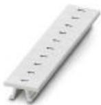
Zack marker strip, Strip, white, labeled, can be labeled with: CMS-P1-PLOTTER, printed horizontally: Identical numbers 1 or 2, etc. up to 100, mounting type: snap into tall marker groove, for terminal block width: 5.2 mm, lettering field size: 5.15 x 10.5 mm, Number of individual labels: 10
