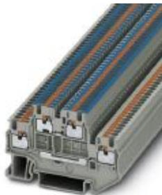
Double-level terminal block, connection method: Push-in connection, cross section: 0.14 mm<sup>2</sup> - 1.5 mm<sup>2</sup>, AWG: 26 - 14, width: 3.5 mm, color: gray, mounting type: NS 35/7,5, NS 35/15
