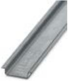
DIN rail, unperforated, Standard profile, width: 35 mm, height: 7.5 mm, acc. to EN 60715, material: Steel, galvanized, length: 2000 mm, color: silver
