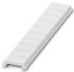
Zack Marker strip, flat, Strip, white, unlabeled, can be labeled with: PLOTMARK, CMS-P1-PLOTTER, mounting type: snap into flat marker groove, for terminal block width: 3.5 mm, lettering field size: 3.5 x 5.2 mm, Number of individual labels: 10
