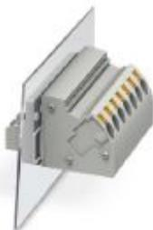
Panel feed-through terminal block, connection method: Push-in spring connection, Slip-on connection, number of positions: 1, load current: 18 A, cross section: 0.2 mm<sup>2</sup> - 4 mm<sup>2</sup>, connection direction of the conductor to plug-in direction: 45 °, width: 8.1 mm, color: gray
