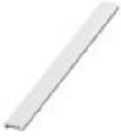
Zack Marker strip, flat, can be ordered: Strip, white, labeled according to customer specifications, mounting type: snap into flat marker groove, for terminal block width: 8 mm, lettering field size: 5.15 x 8.15 mm, Number of individual labels: 10
