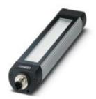
LED machine light, 24 V DC, emission angle 40  $^{\circ}$ /80  $^{\circ}$ , color temperature 5000 K, length 190 mm, diameter 40 mm, M12 connector, Light housing: Anodized aluminum, Pane: Single-pane safety glass (ESG, thermally toughened float glass), pivoting, resistant to coolants and lubricants
