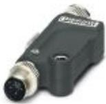
Axioline E IO-Link/analog converter for connecting an analog actuator, 0 V ... 10 V, M12 fast connection technology, straight version
