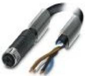
Power cable, 4-position, PUR halogen-free, black-gray RAL 7021, free cable end, on Socket straight M12, coding: T, cable length: 10 m, For direct current up to 12 A/63 V
