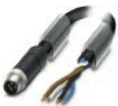
Power cable, 4-position, PUR halogen-free, black-gray RAL 7021, Plug straight M12, coding: T, on free cable end, cable length: 1 m, For direct current up to 12 A/63 V
