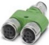
Y distributor, 4-position, Plug straight M12 SPEEDCON, coding: A, on Socket straight M12 SPEEDCON, coding: A, PIN 2+4 bridged and Socket straight M12 SPEEDCON, coding: A, PIN 2+4 bridged, Thread M12 socket not rotatable
