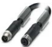
Power cable, 4-position, PUR halogen-free, black-gray RAL 7021, Plug straight M12, coding: T, on Socket straight M12, coding: T, cable length: 1 m, For direct current up to 12 A/63 V
