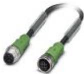
Sensor/actuator cable, 3-position, Variable cable type, Plug straight M12, coding: A, on Socket straight M12, coding: A, cable length: Free input (0.2 ... 40.0 m)
