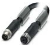
Power cable, 4-position, PUR halogen-free, black-gray RAL 7021, Plug straight M12, coding: T, on Socket straight M12, coding: T, cable length: 2 m, For direct current up to 12 A/63 V
