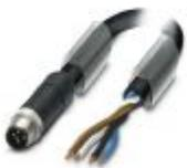
Power cable, 4-position, PUR halogen-free, black-gray RAL 7021, Plug straight M12, coding: T, on free cable end, cable length: 2 m, For direct current up to 12 A/63 V
