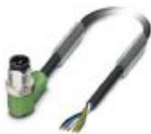
Sensor/actuator cable, 5-position, Variable cable type, Plug angled M12, coding: A, on free cable end, cable length: Free input (0.2 ... 40.0 m)
