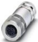
Data connector, PROFIBUS, INTERBUS, 5-position, shielded, Socket straight M12, Coding: B, Screw connection, knurl material: Zinc die-cast, nickel-plated, cable gland Pg9, external cable diameter 6.5 mm ... 8.5 mm
