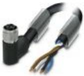
Power cable, 4-position, PUR halogen-free, black-gray RAL 7021, free cable end, on Socket angled M12, coding: T, cable length: 5 m, For direct current up to 12 A/63 V
