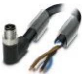
Power cable, 4-position, PUR halogen-free, black-gray RAL 7021, Plug angled M12, coding: T, on free cable end, cable length: 5 m, For direct current up to 12 A/63 V
