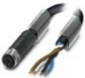
Power cable, 4-position, PUR halogen-free, black-gray RAL 7021, free cable end, on Socket straight M12, coding: T, cable length: 5 m, For direct current up to 12 A/63 V
