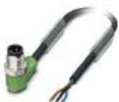
Sensor/actuator cable, 3-position, Variable cable type, Plug angled M12, coding: A, on free cable end, cable length: Free input (0.2 ... 40.0 m)
