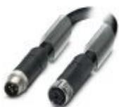
Power cable, 4-position, PUR halogen-free, black-gray RAL 7021, Plug straight M12, coding: T, on Socket straight M12, coding: T, cable length: 10 m, For direct current up to 12 A/63 V
