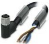
Power cable, 4-position, PUR halogen-free, black-gray RAL 7021, free cable end, on Socket angled M12, coding: T, cable length: 2 m, For direct current up to 12 A/63 V
