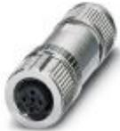
Connector, Universal, 5-position, shielded, Socket straight M12, Coding: B, Push-in connection, knurl material: Zinc die-cast, nickel-plated, external cable diameter 4 mm ... 8 mm
