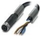
Power cable, 4-position, PUR halogen-free, black-gray RAL 7021, free cable end, on Socket straight M12, coding: T, cable length: 1 m, For direct current up to 12 A/63 V
