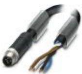
Power cable, 4-position, PUR halogen-free, black-gray RAL 7021, Plug straight M12, coding: T, on free cable end, cable length: 10 m, For direct current up to 12 A/63 V
