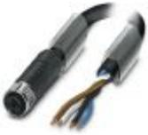
Power cable, 4-position, PUR halogen-free, black-gray RAL 7021, free cable end, on Socket straight M12, coding: T, cable length: 2 m, For direct current up to 12 A/63 V
