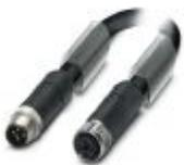
Power cable, 4-position, PUR halogen-free, black-gray RAL 7021, Plug straight M12, coding: T, on Socket straight M12, coding: T, cable length: 0.3 m, For direct current up to 12 A/63 V
