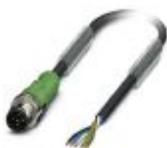
Sensor/actuator cable, 5-position, Variable cable type, Plug straight M12 SPEEDCON, coding: A, on free cable end, cable length: Free input (0.2 ... 40.0 m)
