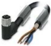
Power cable, 4-position, PUR halogen-free, black RAL 9005, shielded (Advanced Shielding Technology), free cable end, on Socket angled M12, coding: T, cable length: 1.5 m, For direct current up to 12 A/63 V
