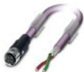
Bus system cable, PROFIBUS (12 Mbps), 2-position, PUR halogen-free, violet RAL 4001, shielded, free cable end, on Socket straight M12 SPEEDCON, coding: B, cable length: Free input (0.2 ... 40.0 m)
