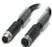
Power cable, 4-position, PUR halogen-free, black-gray RAL 7021, Plug straight M12, coding: T, on Socket straight M12, coding: T, cable length: 5 m, For direct current up to 12 A/63 V
