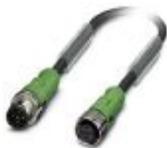
Sensor/actuator cable, 5-position, Variable cable type, Plug straight M12 SPEEDCON, coding: A, on Socket straight M12 SPEEDCON, coding: A, cable length: Free input (0.2 ... 40.0 m)
