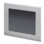
Touch panel with 38.1 cm/15" TFT-display (analog resistive (polyester)), 1024 x 768 pixel(s) (XGA), 65536 colors, Arm9™, 200 MHz, 2x USB host 2.0, 1 x Ethernet (10/100 Mbps), RJ45, Windows CE 5.0 and user software: MicroBrowser. (bus system: without)
