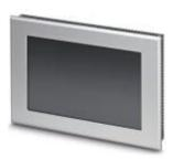
Touch panel with 22.9 cm/9" TFT-display (analog resistive (polyester)), 800 x 480 pixel(s) (WVGA), 65536 colors, Arm9™, 200 MHz, 2x USB host 2.0, 1 x Ethernet (10/100 Mbps), RJ45, Windows CE 5.0 and user software: MicroBrowser. (bus system: without)
