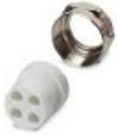
Single screw connection Pg21, made of metal, consisting of rubber seal with a long hole and pressure screw, for type 2-4 housings, cable [mm] 20 x 7 mm (for flat-ribbon cable)
