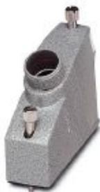
Metal sleeve housing, powder-coating, locking screws with knurled head, type 3, cable screw connection Pg21
