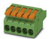
PCB connector, nominal current: 41 A, rated voltage (III/2): 1000 V, nominal cross section: 6 mm², number of positions: 5, pitch: 7.62 mm, connection method: Push-in spring connection, color: green, contact surface: Tin
