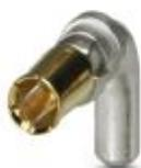
POWER contact, for D-SUB combination inserts, for PCB assembly, socket, angled, rated current 40 A, gold-plated
