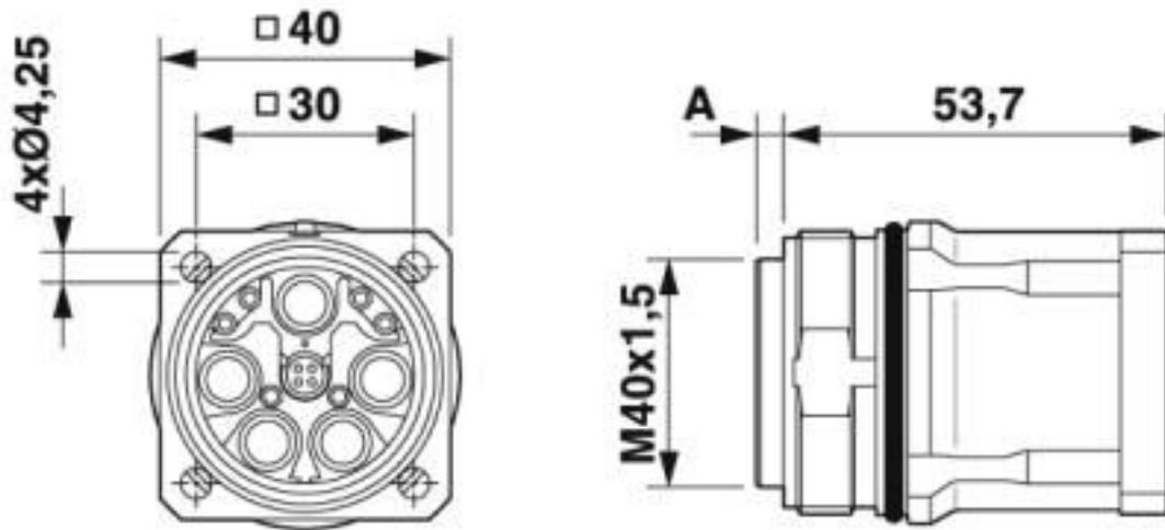
Pin version: dimension A = 3.8 mm, socket version: dimension A = 0.15 mm
