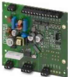
The EV-CC-AC1-M3-CC-SER-PCB charging controller as a PCB for charging electric vehicles on a 3-phase AC power grid according to IEC 61851-1, Mode 3. Optimized for charging stations with permanently mounted Vehicle Connector. All charging functions and comprehensive configuration settings are already integrated.
