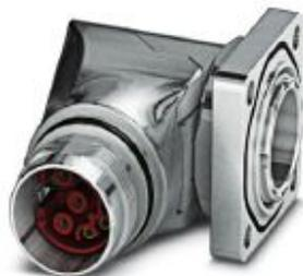
Device connector, front mounting, angled rotatable, for standard and SPEEDCON interlock, M17, number of positions: 8, type of contact: Socket, Axial O-ring, 4x Ø2,7, shielded: yes, flange dimensions: 25.75 mm x 25.75 mm, number of positions: 8, connection method: Crimp connection
