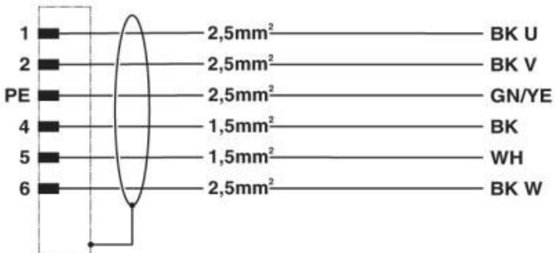
Contact assignment of M23 plugs/sockets
