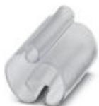
Conductor marker carrier, transparent, unlabeled, mounting type: slide-on, cable diameter range: 10 ... 14 mm, lettering field size: 23 x 4 mm
