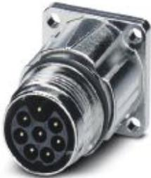
Device connector, front mounting, straight, for standard and SPEEDCON interlock, M17, number of positions: 5+PE, type of contact: Pin, Axial O-ring, 4x Ø2,7, shielded: yes, flange dimensions: 21.6 mm x 21.6 mm, number of positions: 6, connection method: Crimp connection
