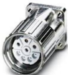
Device connector, front mounting with knurled nut, straight, Screw locking, M23, number of positions: 4+3+PE, type of contact: Socket, Axial O-ring, 4x Ø 3.2, shielded: yes, flange dimensions: 26 mm x 26 mm, cable diameter range: 0 mm ... 0 mm, number of positions: 8, connection method: Crimp connection
