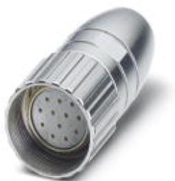
Cable connector, straight, shielded: yes, Screw locking, M23, No. of pos.: 12, type of contact: Socket, Crimp connection
