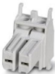
Contact insert, Contact insert, housing material: PA 6.6, number of positions: 2, nom. voltage: 400, rated current: 20 A, Connection method: Screw connection, Type of contact: Socket. Connectors may only be connected/disconnected when under no load.
