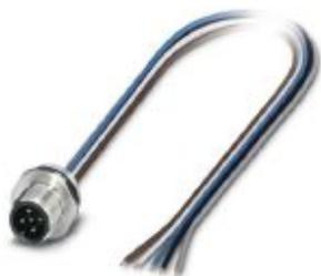
Sensor/actuator flush-type plug, 5-pos., M12, A-coded, front/screw mounting with Pg9 thread, with 0.5 m TPE litz wire, 5 x 0.34 mm<sup>2</sup>, stainless steel version
