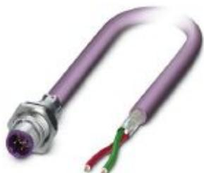
Bus system flush-type plug, PROFIBUS, 2-pos., M12, shielded, B-coded, rear/screw mounting with M16 thread, with 1 m bus cable, 2 x 0.25 mm<sup>2</sup>
