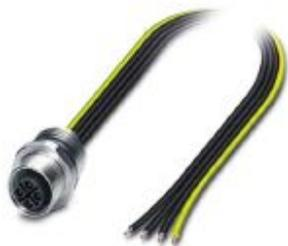
Flush-type connector, Power, 4-position, Socket, M12, S power, Front mounting, M16 x 1.5, Individual wires, cable length: 0.5 m, 1.31 mm<sup>2</sup>, UL/cUL stranded hook-up wire
