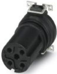
Flush-type connector, 4-position, Socket, straight, M12, D-coded, PCB mounting, SMD
