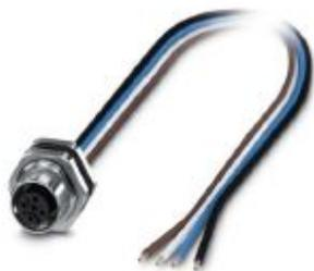
Flush-type connector, Universal, 5-position, Socket, M12, B-coded, Rear mounting, M16 x 1.5, Individual wires, cable length: 0.5 m, 0.34 mm², TPE litz wire
