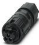
Circular connectors (cable-side), Range of articles: PRC, Connector, housing material: PPE, color: black, number of positions: 3, min. conductor cross section: 1.5 mm<sup>2</sup>, max. conductor cross section: 6 mm<sup>2</sup>, nom. voltage: 690 V AC, rated current: 35 A, Connection method: Screw connection, Type of contact: Pin, min. cable diameter: 8 mm, max. cable diameter: 21 mm
