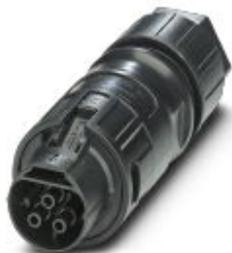
Circular connectors (cable-side), Range of articles: PRC, Coupler connector, type: Can only be released with a tool, housing material: PPE, color: black, number of positions: 3, min. conductor cross section: 1.5 mm<sup>2</sup>, max. conductor cross section: 6 mm<sup>2</sup>, nom. voltage: 690 V AC, rated current: 35 A, Connection method: Screw connection, Type of contact: Socket, min. cable diameter: 16 mm, max. cable diameter: 21 mm. Variant for release with a tool
