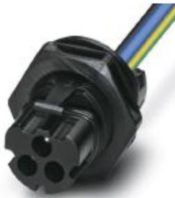
Circular connectors (device-side), Range of articles: PRC, Device connector, rear mounting, housing material: PPE, color: black, number of positions: 3, max. conductor cross section: 2.5 mm<sup>2</sup>, nom. voltage: 690 V AC, rated current: 24 A, Connection method: Crimp connection, Type of contact: Pin, cable length: 150
