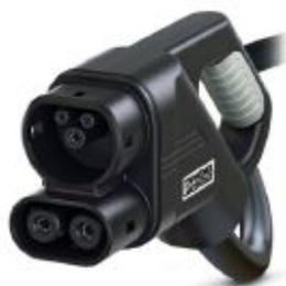
DC charging cable, with vehicle charging connector and open cable end, Housing color black-gray, For charging electric vehicles (EV) with direct current (DC), for installation at charging stations for electromobility (EVSE), CCS type 2, Combined Charging System, IEC 62196-3, 125 A / 1000 V (DC), D-Line 1.0, "PHOENIX CONTACT" logo, cable: 4.5 m, black, straight
