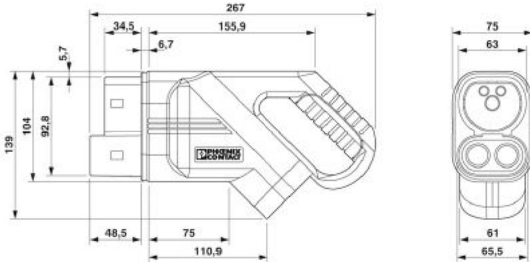
Ensure that the vehicle connector is placed in an appropriate resting position that ensures a minimum protection rating of IP24 in accordance with IEC 61851-1 for the entire time between charging. Use the dimensions of the vehicle connector to create this type of resting position. Detailed specifications can also be found in the download area.
