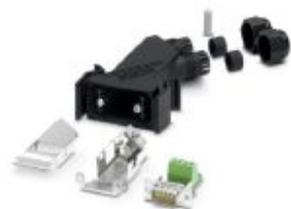
D-SUB connector, degree of protection: IP67, number of positions: 9, material: PA, connection method: Screw connection, connection cross section: AWG 26- 16, cable outlet: Angled, with integrated termination resistor, size of housing: 1, color: black
