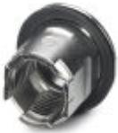
M12 threaded sleeve with tolerance-compensating function, for straight, THR solderable M12 socket contact inserts. Suitable for 3.1 mm ... 3.9 mm thick front plates.
