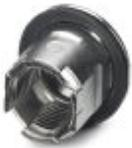
M12 threaded sleeve with tolerance-compensating function, for straight, THR solderable M12 socket contact inserts. Suitable for 2.4 mm ... 3.2 mm thick front plates.
