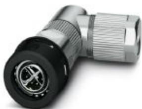
Data connector, Ethernet/PROFINET CAT6<sub>A</sub> (10 Gbps), 8-position, shielded, Plug angled M12 Push-Pull, Coding: X, Crimp connection, knurl material: PA 6.6, external cable diameter 6.5 mm ... 10 mm, without crimp contacts
