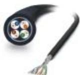
By the meter, Network cable, Ethernet CAT7 (10 Gbps), shielded, PE-X halogen-free, black, 8-wire (4x2xAWG26/7; S/FTP), color single wire: White-blue, white-orange, white-green, white-brown, cable length: 100 m, For railway applications
